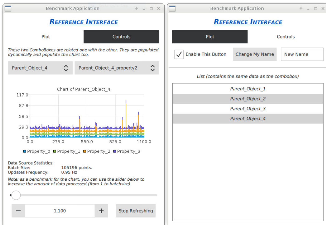
Figure 7.1: QtQuick application has a very modern look and feel and can be styled to look native on most platforms, but shows poor charting performance.
